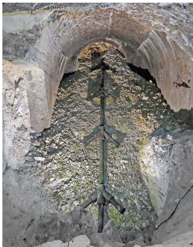
A mock-up of the super-gun shows the slanted booster charge arrangement. Photo Clive Penfold
